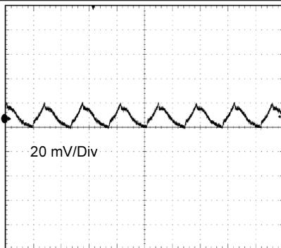
$12\text{ V}_{IN}$ ,  $3.3\text{ V}_{OUT}$  at Full Load, BW = 20 MHz
