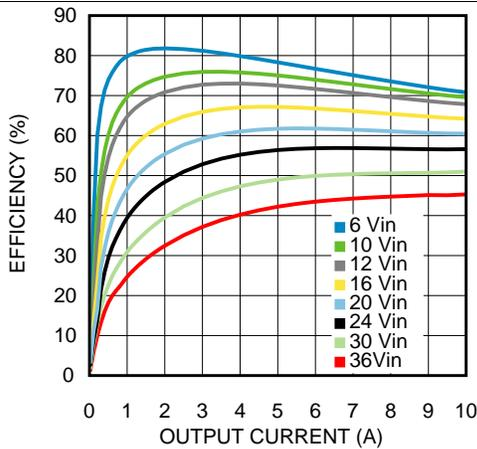
Figure 27. Efficiency 1-V Output at 85°C
