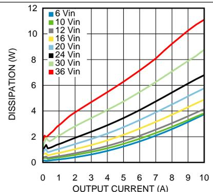
Figure 12. Dissipation 1.2-V Output at 25°C
