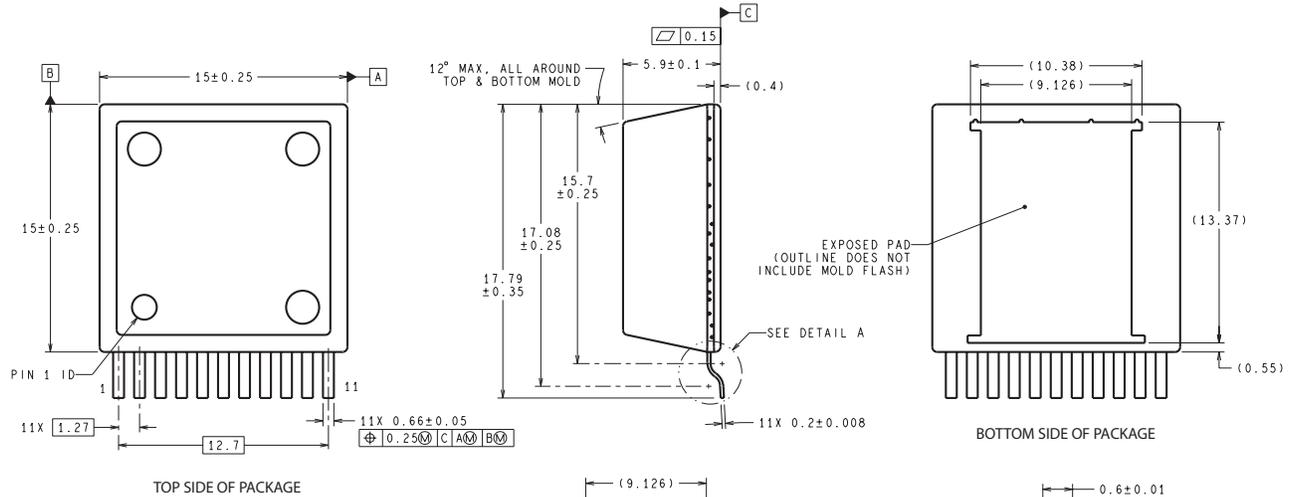
DIMENSIONS ARE IN MILLIMETERS
