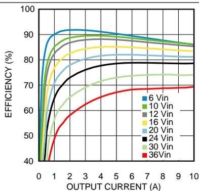
Figure 5. Efficiency 2.5-V Output at 25°C
