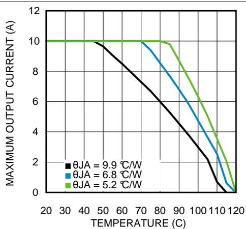
$V_{IN} = 24\text{ V}, V_{OUT} = 5\text{ V}$
