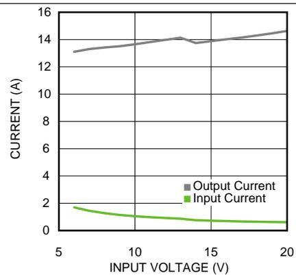
Figure 42. Short Circuit Current vs Input Voltage
