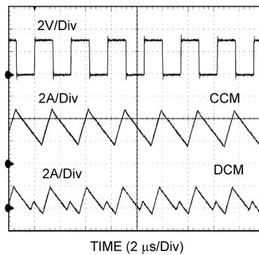
$V_{IN} = 12\text{ V}$ ,  $V_O = 3.3\text{ V}$ ,  $I_O = 3\text{ A} / 0.3\text{ A}$
