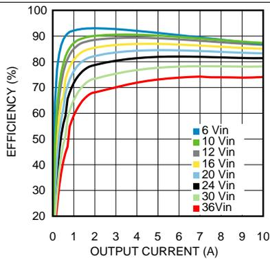
Figure 17. Efficiency 3.3-V Output at 85°C
