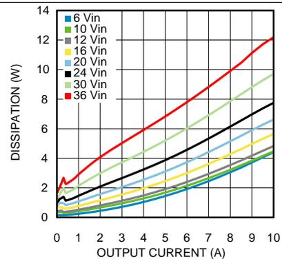
Figure 24. Dissipation 1.5-V Output at 85°C
