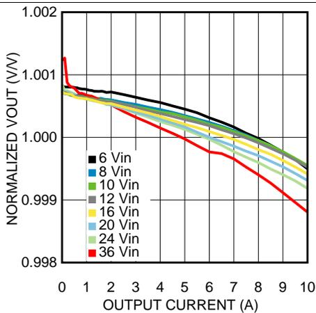
$V_{OUT} = 3.3\text{ V}$
