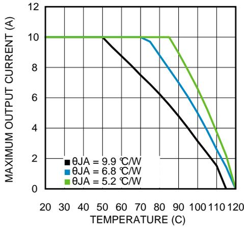
$V_{IN} = 24\text{ V}$ ,  $V_{OUT} = 3.3\text{ V}$
