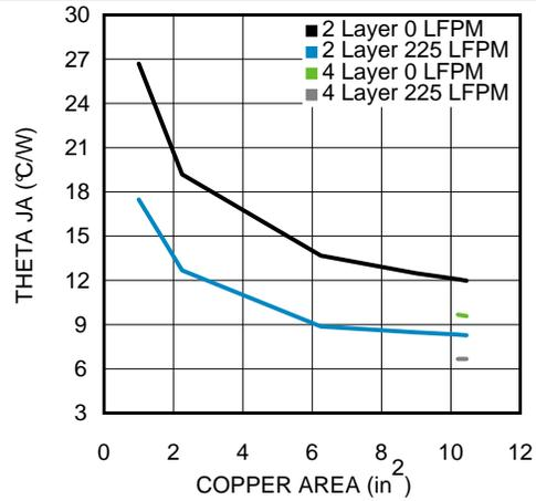
Figure 32.  $R_{J0A}$  vs Copper Heat Sinking Area
