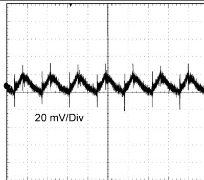
$12\text{ V}_{IN}$ ,  $3.3\text{ V}_{OUT}$  at Full Load, BW = 250 MHz
