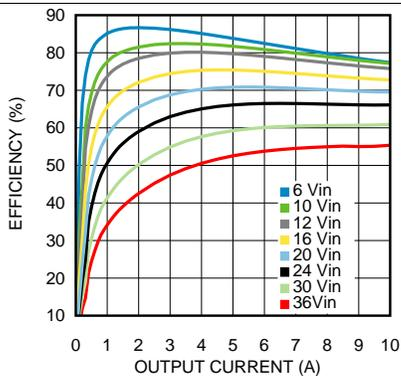
Figure 23. Efficiency 1.5-V Output at 85°C
