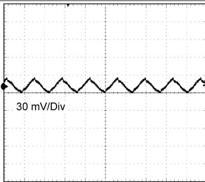
$12\text{ V}_{IN}$ ,  $5\text{ V}_{OUT}$  at Full Load, BW = 20 MHz
