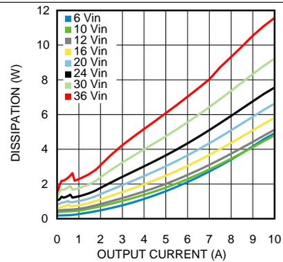
Figure 18. Dissipation 3.3-V Output at 85°C
