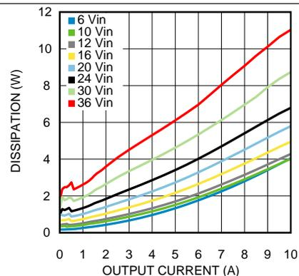
Figure 6. Dissipation 2.5-V Output at 25°C
