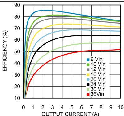
Figure 11. Efficiency 1.2-V Output at 25°C
